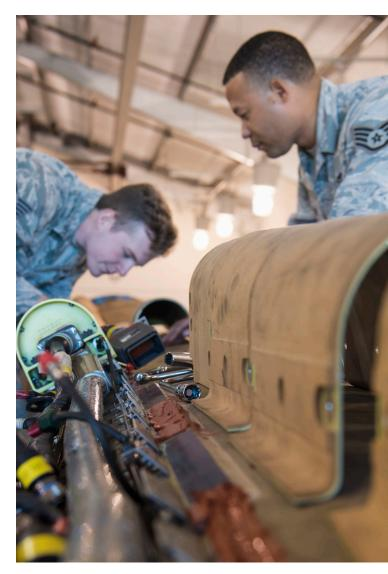
"Staff Sgt. Brandon Dykes connects a telemetry cable on a Minuteman III intercontinental ballistic missile booster," Feb. 3, 2020, Source: U.S. Air Force by Airman 1st Class Aubree Milks
